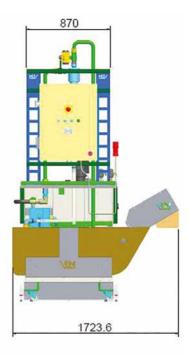
IFDR fine filtration systems are born to take care of the complete management of the coolant, whose role is essential both for the success of the mechanical processing and for the right maintenance of the machine tool.
