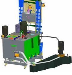
The image shows a complete IFDR 500/25 solution fitted with a delivery pump 20 bar 35 L/min and a delivery pump 70 bar managed by the inverter and the proportional valve, programmed to perform 6 pressure steps at these values: 20, 30, 40, 50, 60, 70 bar with maximum flow rate 40 L/min.
