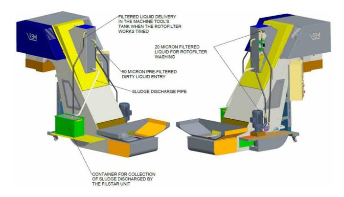
The rotostar solution allows to further reduce the filtration of the rotofilter and is suitable for particularly dusty materials. It is suitable for machine tools that are combined with the A-I rotofilter and that occasionally process materials that tend to make small chips, and there are dispersed powders smaller than  $50 \, \mu m$ .
