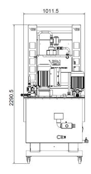
The image shows a complete IFDR 300/20 fine filtration system fitted with a delivery pump 20 bar 35 L/min and a delivery pump 70 bar managed by the inverter and the proportional valve, programmed to perform 6 pressure steps at these values: 20, 30, 40, 50, 60, 70 bar with maximum flow rate 33 L/min.
