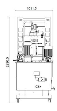
The image shows a complete IFDR 300/25 fine filtration system fitted with a delivery pump 20 bar 35 L/min and a delivery pump 70 bar managed by the inverter and the proportional valve, programmed to perform 6 pressure steps at these values: 20, 30, 40, 50, 60, 70 bar with maximum flow rate 40 L/min.
