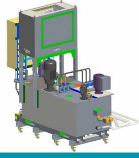
The image shows a complete IFDR 800/25 fine filtration system fitted with a delivery pump 20 bar 35 L/min and a delivery pump 70 bar managed by the inverter and the proportional valve, programmed to perform 6 pressure steps at these values: 20, 30, 40, 50, 60, 70 bar with maximum flow rate 45 L/min, and chiller for coolant's temperature control. This solution is dedicated to lathes with two spindles and 2/3 turrets, which need high and low pressure on the tools.
