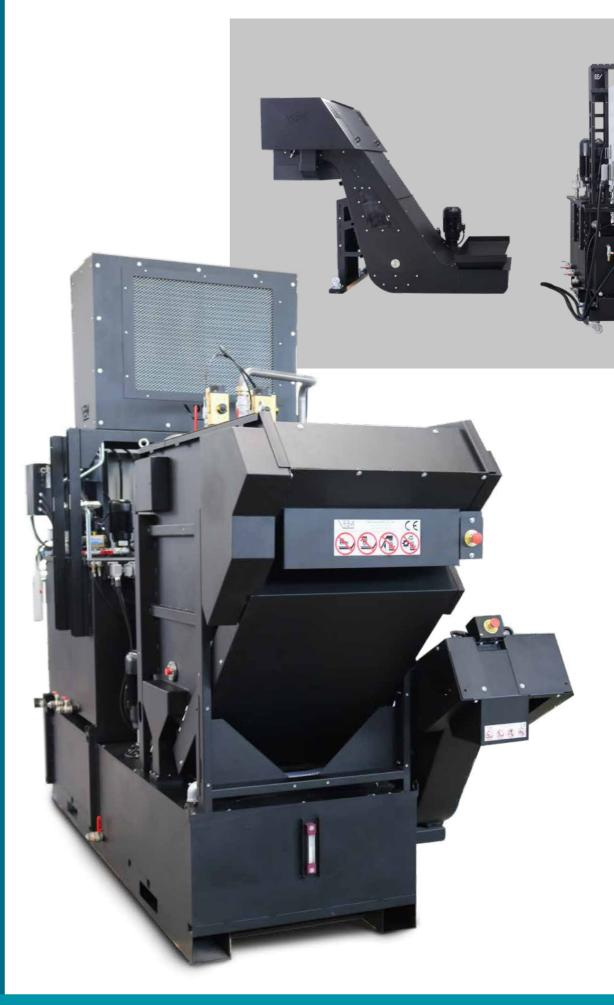
IFDR fine filtration systems are born to take care of the complete management of the coolant, whose role is essential both for the success of the mechanical processing and for the right maintenance of the machine tool.
