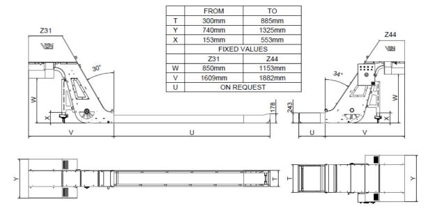
The dimensions T, Y, and X can assume the following values (mm) to adapt the conveyor to the tank of the machine tool.
