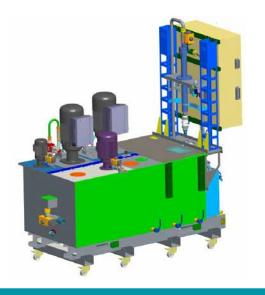
The image shows a complete IFDR 800/32 fine filtration system fitted with DUPLEX system, which guarantees a flow rate from 8 to 85 L/min in the first version and from 18 to 120 L/min in the second one.
