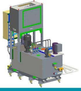
The image shows a complete IFDR 800/25 fine filtration system fitted with a delivery pump 20 bar 35 L/min and a delivery pump 70 bar managed by the inverter and the proportional valve, programmed to perform 6 pressure steps at these values: 20, 30, 40, 50, 60, 70 bar with maximum flow rate 45 L/min, and chiller for coolant's temperature control. This solution is dedicated to lathes with two spindles and 2/3 turrets, which need high and low pressure on the tools.
