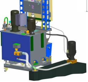
The image shows a complete IFDR 300/25 fine filtration system fitted with a delivery pump 20 bar 35 L/min and a delivery pump 70 bar managed by the inverter and the proportional valve, programmed to perform 6 pressure steps at these values: 20, 30, 40, 50, 60, 70 bar with maximum flow rate 40 L/min.
