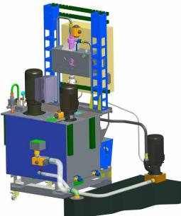
The image shows a complete IFDR 300/20 fine filtration system fitted with a delivery pump 20 bar 35 L/min and a delivery pump 70 bar managed by the inverter and the proportional valve, programmed to perform 6 pressure steps at these values: 20, 30, 40, 50, 60, 70 bar with maximum flow rate 33 L/min.
